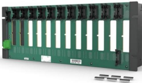
The EMC-DB01 Evolution Mounting Chassis, Divisible Bus, REAR mounting rail provides mounting space for up to twelve (12) evolution modules within the same space as an MMU. The EMC chassis replaces MMU11 or MMU21 Module Mounting Units. The chassis has been designed so that I/O cables originally attached to the MMU can be attached in the exact same location once the EMC has replaced the MMU.
