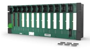
The EMC-DB01 Evolution Mounting Chassis, Divisible Bus, REAR mounting rail provides mounting space for up to twelve (12) evolution modules within the same space as an MMU. The EMC chassis replaces MMU11 or MMU21 Module Mounting Units. The chassis has been designed so that I/O cables originally attached to the MMU can be attached in the exact same location once the EMC has replaced the MMU.
