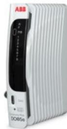
The DO05e digital output module provides eight (8), CH-2-CH isolated electromechanical relay contact outputs. The electromechanical relay contacts are capable of handling up to 3.0 A. The module executes at a 1-msec cycle and has an average response time of 0.5 msec based on when the command is received from the controller
