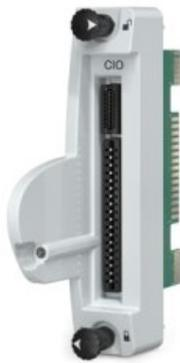
The EMB01S-CIO Evolution Module Base provides the mounting of an AD11e Analog Drive module to an EMC-\_B0x Evolution Mounting Chassis. The base connects the I/O module to the HN800 I/O bus and the I/O cable to the field termination.
