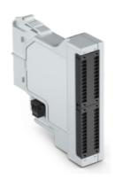
The HDT-UAI-01 High-Density Termination module is used to terminate field wiring for up to 16 I/O Channels to the back side of an EMC-B0x Evolution Mounting Chassis. The HDT is installed on the back side of an EMC using an HDT-BRK-01 mounting bracket assembly. The HDT-UAI-01 provides header connectors for four (4) pluggable 12-PT Terminal Blocks (which are sold separately). The HDT-UAI-01 also provides a 2-PT Terminal Block for the connection of Field I/O power.
