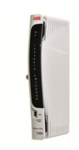
The DIO4 digital input module processes up to 16 individual Digital Input signals. Each channel is individually CH-2-CH isolated and supports 48 VDC inputs. FC 221 (I/O Device Definition) sets DI module operating parameters and each input channel is configured using FC 224 (Digital Input CH) to set input channel parameters such as alarm state, debounce period, etc.
