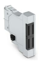
The HDT-XIO-01 High-Density Termination module is used to terminate field wiring for up to 16 I/O Channels to the back side of an EMC-B0x Evolution Mounting Chassis. The HDT is installed on the back side of an EMC using an HDT-BRK-01 Bracket mounting assembly. The HDT-XIO-01 provides header connectors for four (4) pluggable 8-PT Terminal Blocks (which are sold separately). The HDT-XIO-01 also provides a 2-PT Terminal Block for the connection of Field I/O power.
