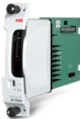
The AI16ev Universal Analog Input module processes up to sixteen (16) high-level, CH-2-CH isolated, analog input field signals. Each channel is independently configurable for high-level (4 to 20 mA or 1 to +5 VDC), RTD, mV, and TC analog input signal ranges.
