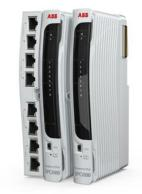
The SD Series SPC600 are the newest additions to the Symphony Plus controller family. SPC600 controller features include; modular high-density design, low energy consumption, flexible DIN-Rail column or row mounting, and extreme operating temperature range (-40 to +70 degC).
