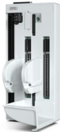
The VBR11e-EPD mounting base is for the Redundant Mixed I/O (AD11e) Analog I/O (AI12e, FI12e, AO02e), and Digital I/O (DI06e, DO01e, DO05e) modules and the (PI01e) Pulse input Module. The base is designed to accommodate field signals that are externally powered or are differential inputs.
