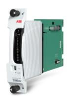
The SI06ev SOE Input module processes up to 16, CH-2-CH isolated, digital input field signals for Sequence of Events reporting. Each channel is independently configurable for 24 / 48 / 110 / 125 VDC, or 100 / 120 VAC input signal voltages.
