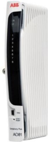
The AO01 Analog Output module processes up to 16 high level, group isolated, analog output field signals. Each channel is independently configurable for either 4 to 20 mA or 1 to +5 VDC ranges. FC 221 (I/O Device Definition) sets AO module operating parameters and each output channel is configured using FC 223 (Analog Output CH) to set individual output channel parameters such as engineering units, High/Low alarm limits, default value in event of loss of communication with controller, etc.
