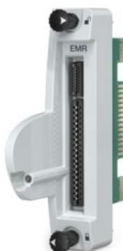
The EMB01S-EMR Evolution Module Base provides the mounting of a DO05e EMR Digital Output module to an EMC-\_B0x Evolution Mounting Chassis. The base connects the I/O module to the HN800 I/O bus and the I/O cable to the field termination.
