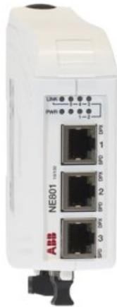
The NE801 is an Industrial Ethernet 5-port switch. All ports support auto-negotiation, but DIP switches also allow speed and duplex configuration of any individual TX port. It is also possible to set up one port to monitor traffic to/from the switch. The NE801 has been designed to meet high industrial specifications, providing very high dependability in harsh environmental conditions.
