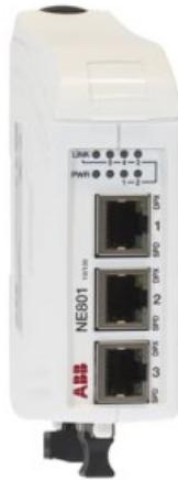
The NE801 is an Industrial Ethernet 5-port switch. All ports support auto-negotiation, but DIP switches also allow speed and duplex configuration of any individual TX port. It is also possible to set up one port to monitor traffic to/from the switch. The NE801 has been designed to meet high industrial specifications, providing very high dependability in harsh environmental conditions.
