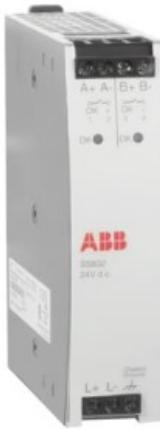
The Voting Units SS823 and SS832 have been specifically designed to be employed as control units within a redundant power supply configuration. The output connections from two Power Supply Units are connected to the Voting Unit.
