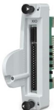
The EMB01S-EMR Evolution Module Base provides the mounting of an AI12e, AO02e, DI06e, or DO01e I/O module to an EMC-\_B0x Evolution Mounting Chassis. The base connects the I/O module to the HN800 I/O bus and the I/O cable to the field termination.
