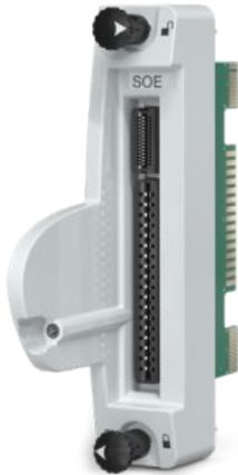
The EMB01S-SOE Evolution Module Base provides the mounting of a DI06e to an EMC-\_B0x Evolution Mounting Chassis. The base connects the DI06e I/O module to NKSD01-xx or NKTST01-xx I/O cables that are connected to NTDI01 or NTST01 field termination units for SOE applications.
