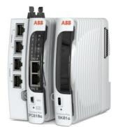
The SPC810eK01 is a SINGULAR Symphony Plus controller that mounts to a horizontal DIN-Rail using MB910e base. Controller features include; a modular high-density design, low energy consumption, extreme operating temperature range (-40 to +70 °C), and multiple deployment options of the SPC810e module.
