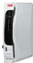
The AI12e Analog Input module processes up to sixteen (16) high-level analog input field signals. Each channel is independently configurable for any of the supported high-level signal ranges.
