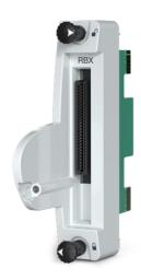
The **EMB01S-RBX** Evolution Module Base for Remote Bus eXtender is used to mount an RBX01e Enhanced Remote Bus eXtender fiber optic repeater module to an EMC Evolution Mounting chassis of Symphony Plus.
