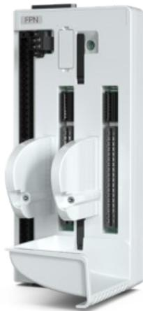
The VBR11e-FPN mounting base is for the Redundant Digital I/O (DI06e, DO01e) modules and the (PI01e) Pulse inut Module. The base is designed to accommodate field signals that are system powered and the (-) Neutral side of power is switched.
