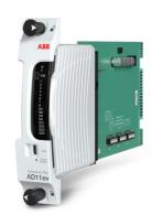
The AD11ev Analog Drive module processes up to thirteen (13) mixed type field signals. The AD11ev provides 4x AI, 2x AO, 3x DI and 4x DO signals.
