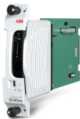
The DO05ev digital output module provides eight (8), CH-2-CH isolated electromechanical relay contact outputs. The electromechanical relay contacts are capable of handling up to 3.0 A. The module executes at 1-msec cycle and has an average response time of 0.5 msec based on when the command is received from the controller.
