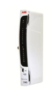
The DIO3 digital input module processes up to 16 individual Digital Input signals. Each channel is individually CH-2-CH isolated and supports 24 VDC inputs. FC 221 (I/O Device Definition) sets DI module operating parameters and each input channel is configured using FC 224 (Digital Input CH) to set input channel parameters such as alarm state, debounce period, etc.
