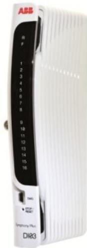
The DI03 digital input module processes up to 16 individual Digital Input signals. Each channel is individually CH-2-CH isolated and supports 24 VDC inputs. FC 221 (I/O Device Definition) sets DI module operating parameters and each input channel is configured using FC 224 (Digital Input CH) to set input channel parameters such as alarm state, debounce period, etc.
