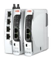
The SPC810eK02 is a REDUNDANT Symphony Plus controller that mounts to a horizontal DIN-Rail using MB910e base. Controller features include; a modular high-density design, low energy consumption, extreme operating temperature range (-40 to +70 °C), and multiple deployment options of the SPC810e module.
